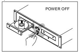
Do not switch off the power when the disc holder is open.
